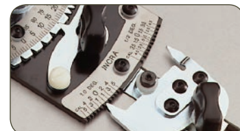
▲ AngleLOCK™ Indexing. Precision angle indexing teeth are laser-cut in solid steel to lock in 364 positive angle stops in 1/2°, 1° or 5° increments over a full 180° range.
