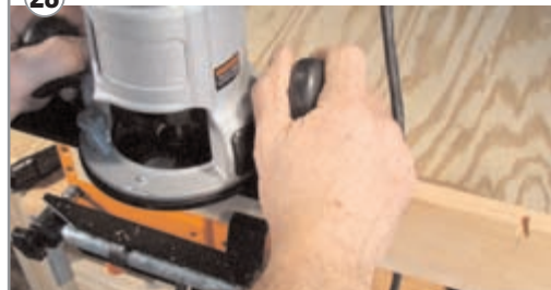
28. Align the layout lines with the centerline in the Top Plate and cut the dovetail sockets.
