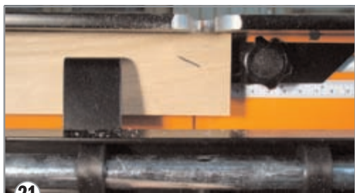
21. Reposition the stop at the 1-3/8-in. position and repeat the process for the second dovetail socket on each rail and stile.
