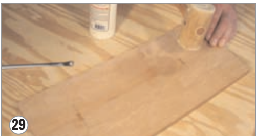
29. Apply glue to the edges of the boards, close the joint, and insert the keys and caps.
