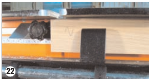
22. Reposition the stop, using the same settings as on the right side , on the left side and repeat the process, placing parts labeled with a 2 against the stop in this position.
