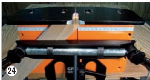
24. Mitered parts Place layout lines for locating the dovetail sockets on one miter. Position the piece in the Enlock Jig with one of the layout lines under the centerline in the Top Plate.
