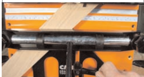
26. From this position, the left and right miters can both be joined. When the first socket has been cut in each piece relocate the Miter Plate for the second socket.
