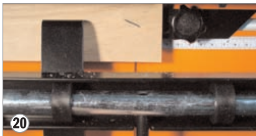
20. Add the Clamp Extension Arm and butt the stiles labeled with a 1 horizontally against the stop and cut a dovetail socket.
