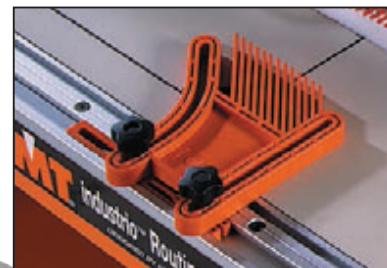
999.501.07_Moulded ABS featherboard setup on the table and in fence slots. In includes nuts, bolts and a plastic slide.
