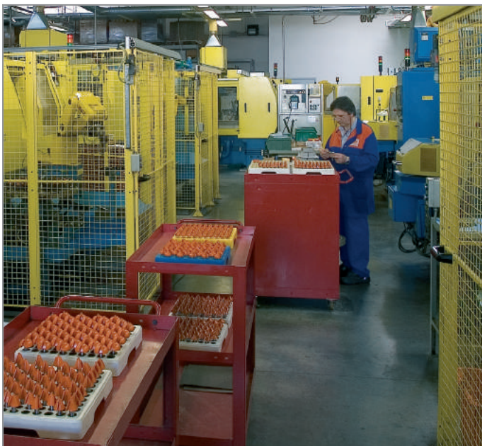
Loading the automated multi-axis CNC sharpening machines.
