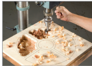
Rough out the interior using a drill press and a 50,8mm Forstner bit.
